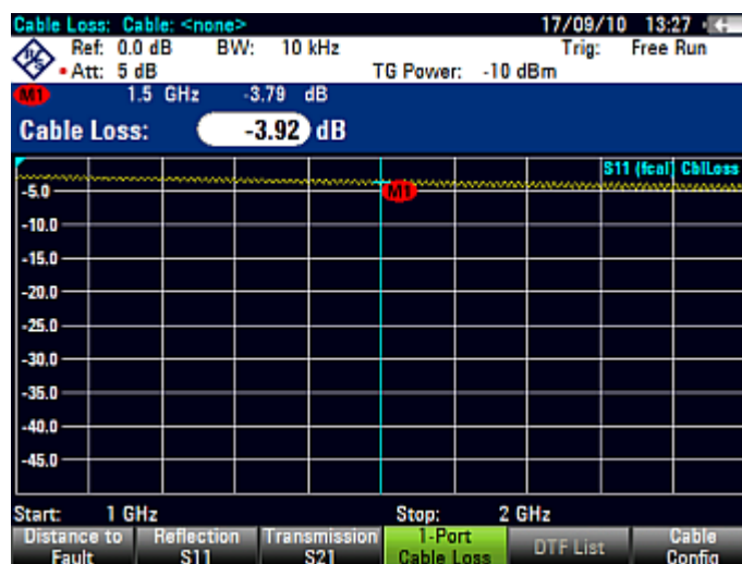
Figure 2-4: Results of a cable loss measurement
